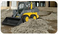
**Skid Steer** for moving piles of ThorTurf around arena.
